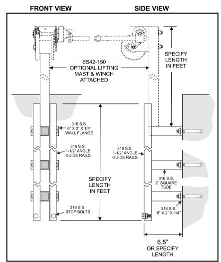
GR-1 guide rails use 316 stainless steel materials for long term duty in harsh water, wastewater, or CSO basin applications.
